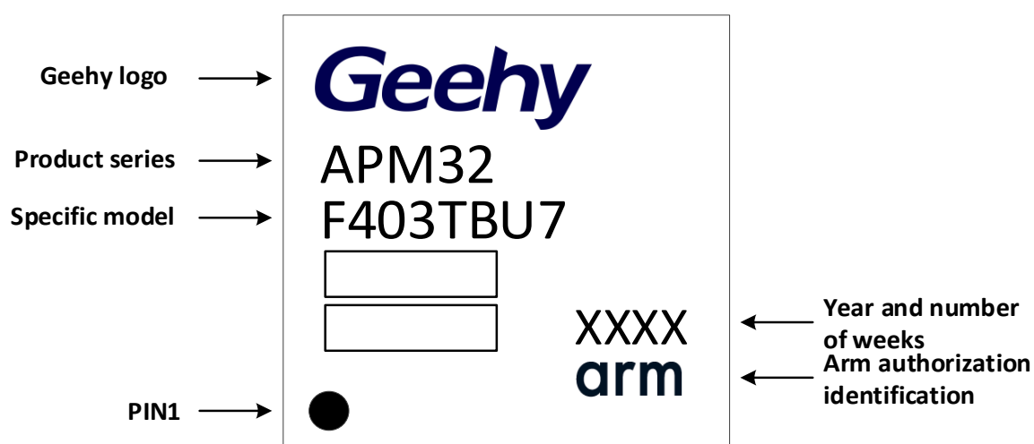
Figure 27 QFN36-36 Pin 6x6mm Identification
