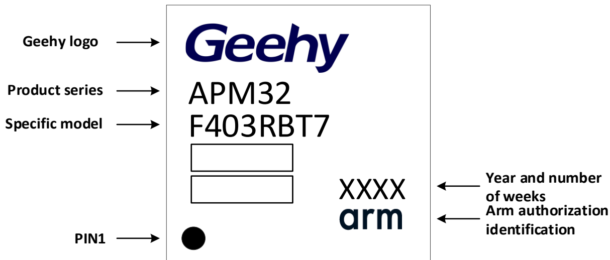
Figure 18 LQFP64 - 64 Pins, 10 x 10mm Package Identification
