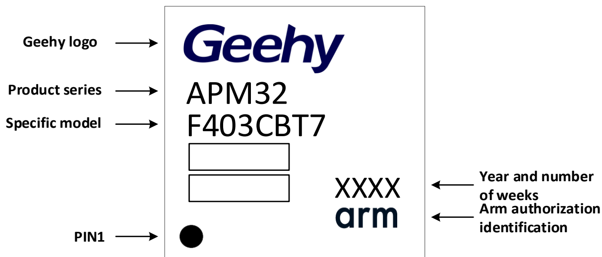
Figure 21 LQFP48 -48 Pins, 7x7mm Identification
